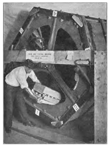
Fig. 49.—Box-testing machine.
